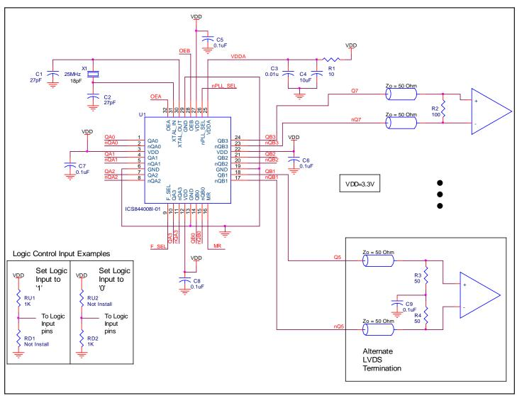
FIGURE 7. ICS844008I-01 SCHEMATIC LAYOUT
