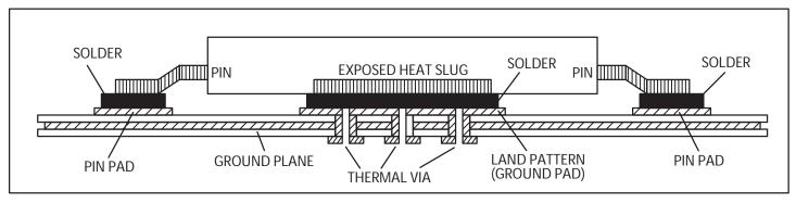
FIGURE 5. ASSEMBLY FOR EXPOSED PAD THERMAL RELEASE PATH -SIDE VIEW (DRAWING NOT TO SCALE)
