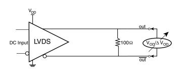
DIFFERENTIAL OUTPUT VOLTAGE SETUP
