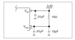
FIGURE 1. POWER SUPPLY FILTERING
