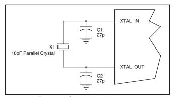
FIGURE 2. CRYSTAL INPUT INTERFACE
